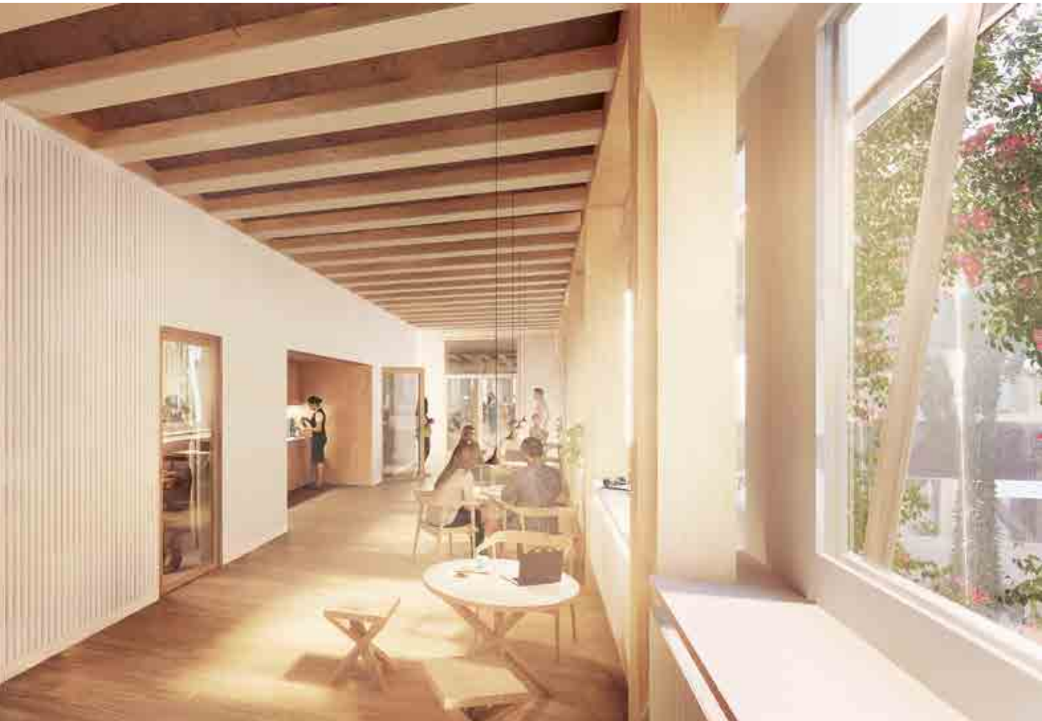
The components for the building were as unprocessed as possible, with plenty of solid and deciduous wood and little laminated timber used.
