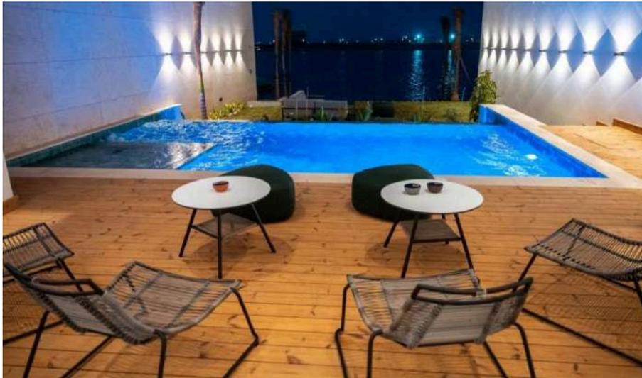
Located near the seaside, an area with high exposure to extreme heat and humid conditions, especially in summer, thermowood was chosen due to its durability and high stability.
