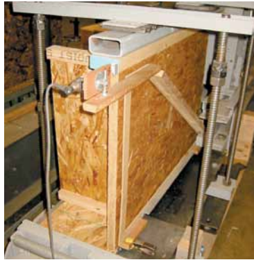
An APA Performance Rated Rim Board sample is evaluated for structural performance at the APA Research Center.
