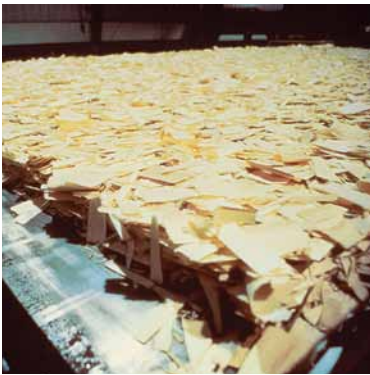
OSB is produced from thin rectangular-shaped wood strands that are formed in a mat.
